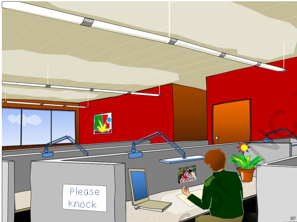
Figure 32 – TAL system with indirect ambient luminaires (illustrated by Yukio Akashi)
